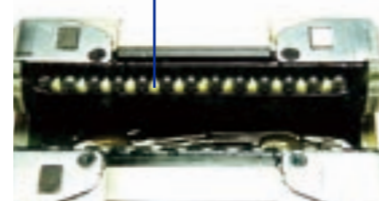
After testing, grease remains without anomalies.
