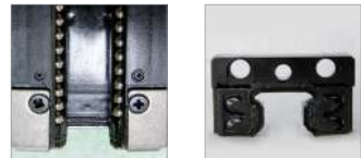
Plastic parts in good condition End seal in good condition
